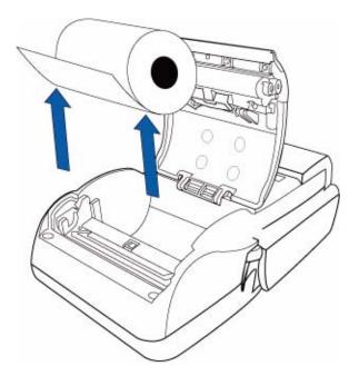
Figure 10 Removing Partial Paper Roll
